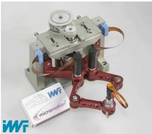
Fig. 1. PARVUS parallel scara-robot [4]
