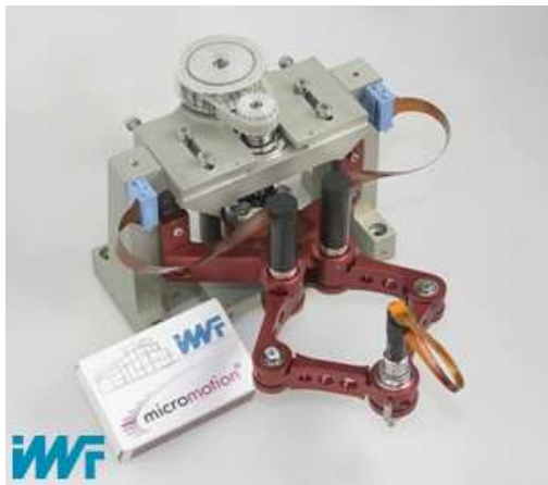
Fig. 1. PARVUS parallel scara-robot [4]
