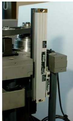
Fig. 7. The linear displacement sensor that have a resolution of 0.1\mu\text{m}
