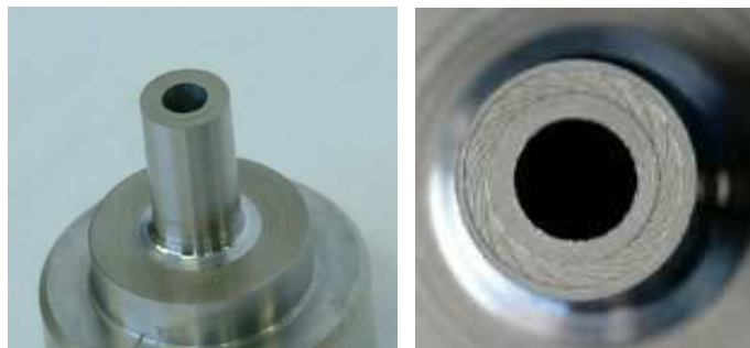
Fig. 9. Manufactured mold for forming the herringbone pattern on the metal substrate
