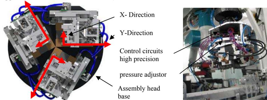
Fig. 4. Illustration of the orientation of the endeffector positioning capabilities (bottom view, left) and a photo of the assembly head prototype within a robot system (right)
