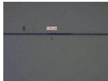
Fig. 8. : Adhesive gap of <math>< 3 \mu\text{m}</math>
