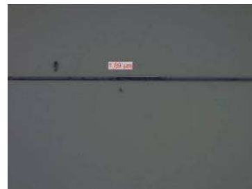
Fig. 8. : Adhesive gap of < 3 µm
