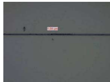
Fig. 8. : Adhesive gap of < 3 \mu\text{m}
