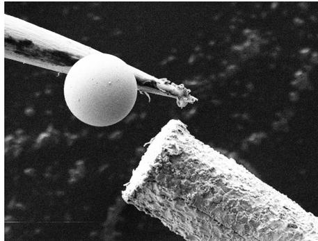
**Fig. 7.** SEM image showing the assembly of the sphere onto the shaft
