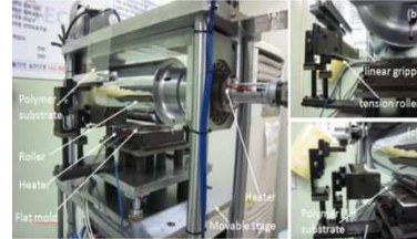
Fig. 7. Photographs of major components
