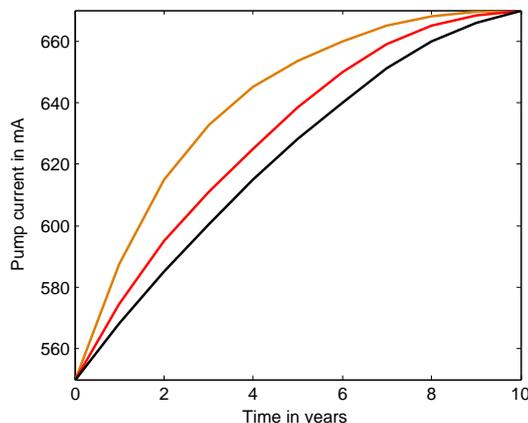
**Fig. 1.** Different aging curves of EDFAs
