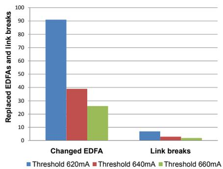
Fig. 3. Number of EDFA outages and link breaks for scenario 2
