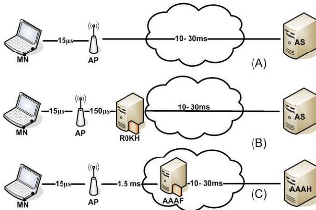
Fig. 6. Experiment of Handover Times in Different Cases
