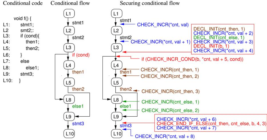
Fig. 6. Securing conditional control flow
