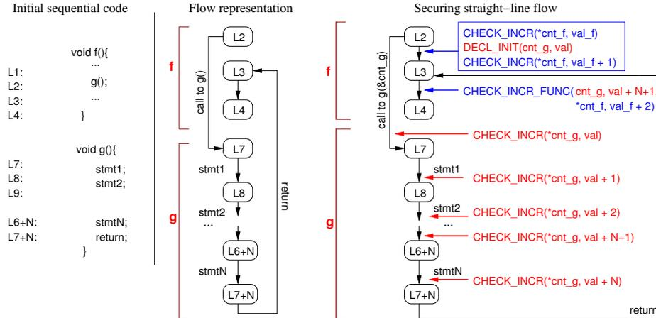
Fig. 5. Securing function call and straight-line flow
