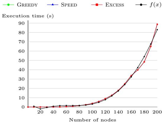
Figure 6: Study of the impact of the number of nodes on the execution time, for random requests between 0 and 100,  $\mathcal{P}_{\text{static}} = 50,000$ , average on 100 tests.
