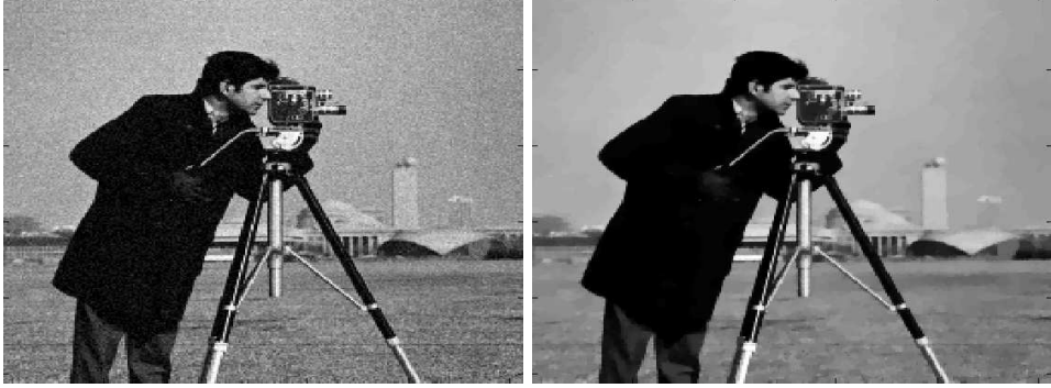
Left: noisy image y^0 . Right: the image \hat{x} estimated minimizing F with FISTA.
