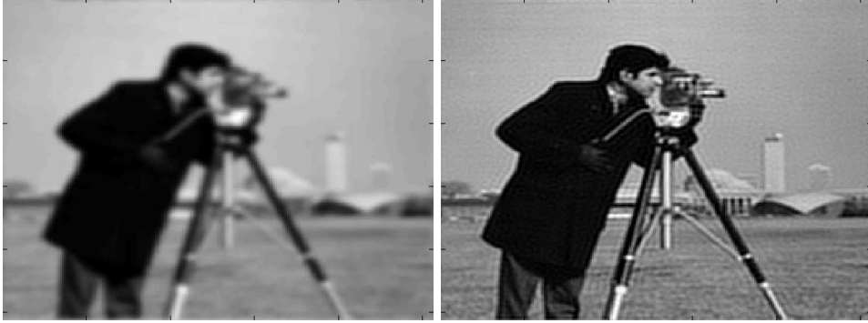
Left: the blurred image y^0 . Right: an image \hat{x} estimated minimizing F with FISTA.
