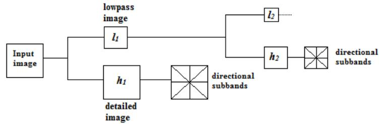
**Fig. 1.** The contourlet filter bank. Images  $l_i$  and  $h_i$  are the lowpass and detailed image, respectively, obtained from the  $i$ th level of decomposition with the LP. In every level of LP decomposition,  $h_i$  is fed into the DFB.
