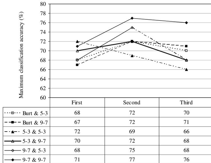
**Fig. 3.** Maximum classification accuracy of the  $k$ -NN classifier for each filter combination at each level of LP decomposition (first, second, third). The first filter of the filter combinations refers to the one used for the LP and the second refers to the one used for the DFB.
