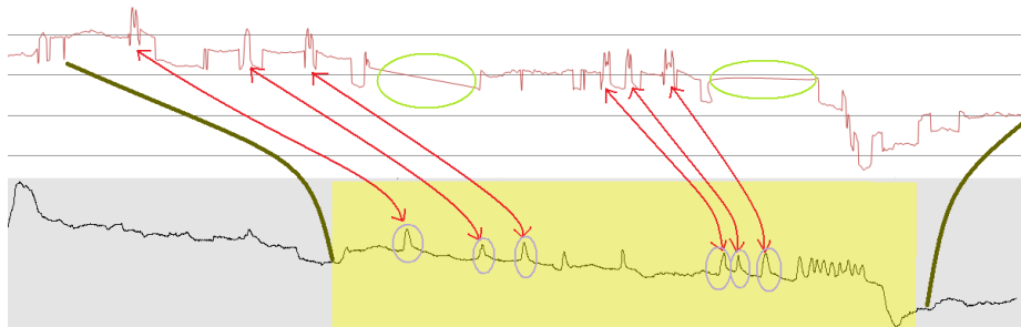
Fig. 4. Comparing recorded results ( first graph ) with EDF stored results ( bottom graph ). In this experiment session, the first three blinks are properly recorded and processed. The following two blinks are missed due processor delay. The next 3 blinks are also properly assessed. The continuous blinking at the end of the session is missed by the application.
