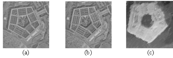
Fig. 4. (a) Left image; (b) right image; (c) the estimated disparity map.
