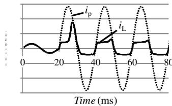
**Fig. 8.** Evolution of current in the circuit,  $i_L$ , under a fault, applied at 20 ms. Prospective current,  $i_p$ , is also shown. Results are taken from [8].
