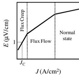
Fig. 3. HTS  $E$ - $J$  qualitative dependence. The  $1 \mu\text{V}/\text{cm}$  criterion defines critical current density,  $J_c$ , below which the material is in the superconducting state. Above  $J_c$  and below normal state, the material is in the mixed state.
