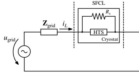
Fig. 2. Resistive superconducting fault current limiter electrical diagram.
