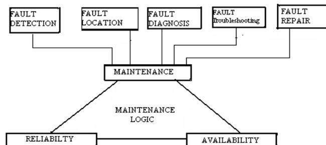
**Fig. 1.** Connections between reliability, maintenance and availability.
