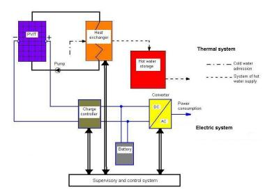
Fig. 3. Block diagram of PV/T system.
