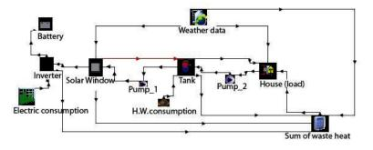
Fig. 4. Block diagram of a PV/T TRNSYS model [21].
