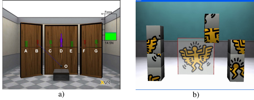
Fig. 3 Virtual reality applications with force sensing. a) The reaching video-game-like application, it will be used for our trials. b) Cubes application, it consists into a 3-dimensional puzzle to be organised by the patients.
