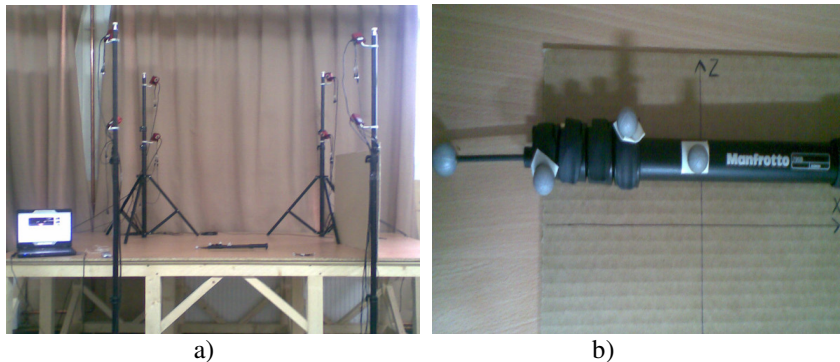
Fig. 1. a) The displacement of the camera; b) The object used to accomplish the measurements.
