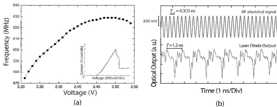
**Fig. 3.** (a) Optoelectronic voltage controlled oscillator. (b) Electro-optical conversion: injection locking at around 0.75 GHz measured in the laser output when a 3 GHz RF signal is injected in the RTD-OEO electrical input port.
