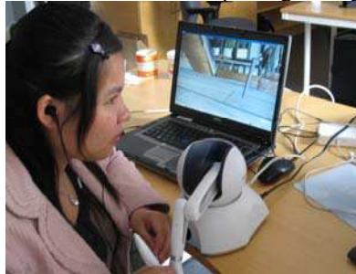
Fig. 3. User interacting with the haptic virtual environment using a PHANTOM Omni force feedback device (source: SensAble Technologies Inc)
