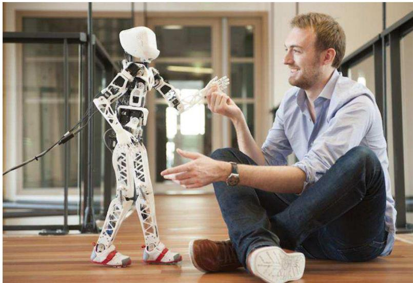
The design of humanoid robots for rich, safe interactions with everyday environments and humans requires techniques for online learning of sensorimotor and social control skills. The open-source 3D-printed humanoid robot Poppy shown here allows systematic experimentation in the integration of such learning methods with adequately designed morphologies (<http://www.poppy-project.org>; photo Inria/H. Raguet).
