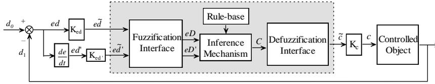
Fig.3: Structure of the fuzzy controller
