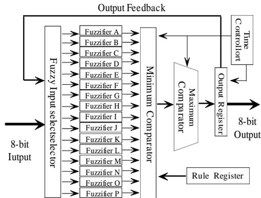
Fig.6: Internal structure of NLX230
