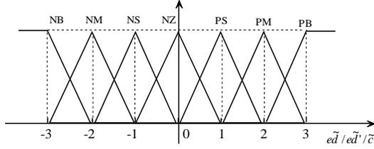
Fig.4: Membership functions of the inputs and output
