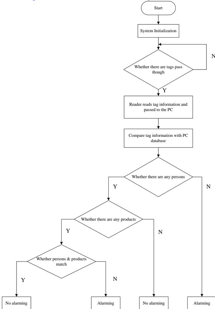
Fig.3: warehouse products monitoring system work flow chart
