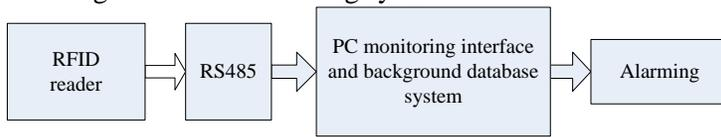
Fig.2: Hardware configuration of monitoring system
