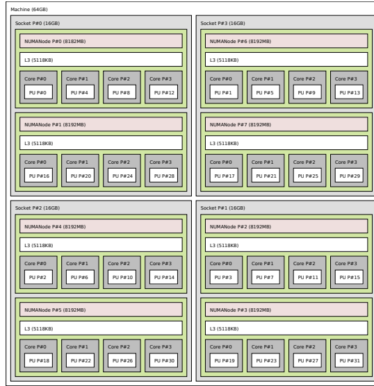
Fig. 5: hwloc output describing the topology of the dell32 multicore machine.
