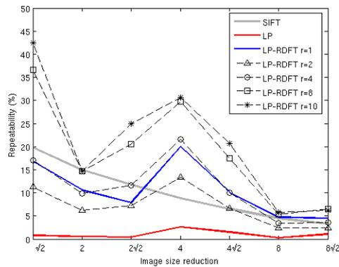
Fig. 6: Repeatability under changes in image scale. The horizontal axis shows the scale factor for smaller scaled images. The letter  $r$  stands for the neighborhood radius for the RDFT. LP-RDFT with a 2D RDFT of radius 10 is the most repeatable under changes in image scale followed by LP-RDFT with a 2D RDFT of radius 8. Relative peaks appear when the scale factor of the test data corresponds to the scale of the pyramid levels. The plots are clearer in color.
