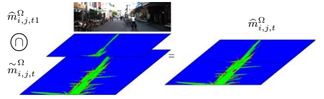
Fig. 7: Merging step of the C-SALM algorithm based on [21]
