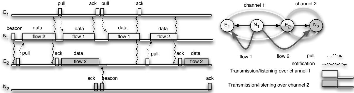
Fig. 6. Pull mechanism and notifications for packet forwarding between nodes  $E_1$  and  $N_2$ .
