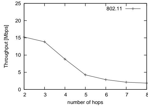
Fig. 2. Throughput vs. number of hops in the single channel case.
