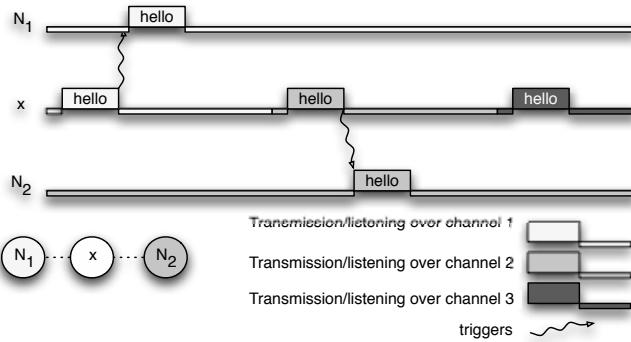
Fig. 8. An example of new node  $x$  joining a molecular mesh network.
