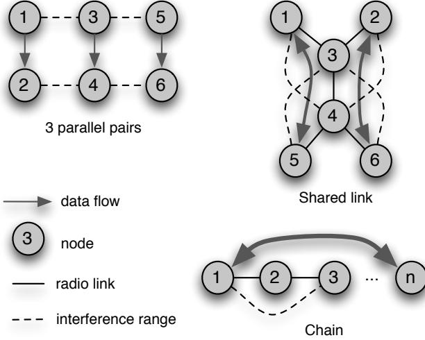
Fig. 10. 3 pairs, shared link, and chain configurations.
