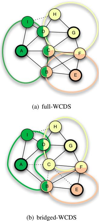
Fig. 2. Examples of a full-WCDS and a bridged-WCDS.
