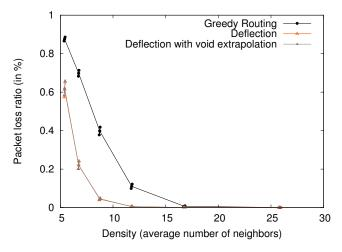
Figure 5: Packet loss under different routing schemes for UDG.
