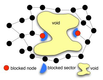
Figure 1: Blocked nodes in greedy geographical routing.
