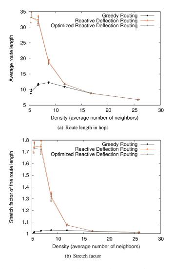
Figure 6: Route length under different routing schemes for UDG.
