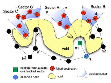
Figure 2: Examples of blocked nodes and blocked sectors.
