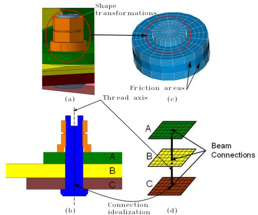
Fig. 2. Example of adaption from DMU to FE analysis model: a) a 3D view of a bolt in a DMU, b) a cutout of a bolt and its neighboring components, c) simplified bolt for detailed stress distribution with friction between plates and discretization with a hexahedral mesh, b) idealized bolt and plates to set up a global model for the bolt as a connector.
