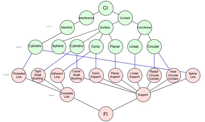
Fig. 6. The taxonomies  $\mathcal{T}_{ci}$  of CIs and  $\mathcal{T}_{fi}$  of FIs derived from  $\mathcal{T}_{ci}$ , partially illustrated.  $\mathcal{T}_{ci}$  is represented in light blue and  $\mathcal{T}_{fi}$  in pink. Dotted lines between the leaves of  $\mathcal{T}_{ci}$  and  $\mathcal{T}_{fi}$  illustrate the multiple functional interpretations that originate leaves of  $\mathcal{T}_{fi}$  from leaves of  $\mathcal{T}_{ci}$ .
