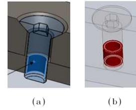
Fig. 4. An example of CI of type interference between a **screw** and an assembly component: a) CI location between the **screw** and the assembly component, b) volume of interference defining their CI.
