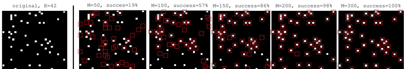
**Fig. 7.** Reconstruction of a sparse input with a real hardware compressive sampler using scattering material and  $P = 3$ . Red squares indicate the pixels identified as active, the original image is shown in the background.
