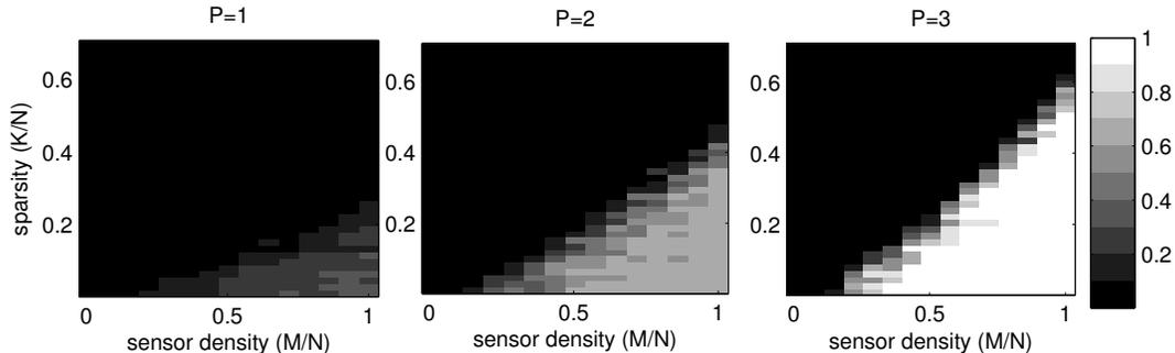
**Fig. 6.** Performance of CS reconstruction of sparse inputs imaged experimentally through our optical setup. Due to the presence of strong noise, only MMV at  $P = 3$  permits reconstruction with high probability.
