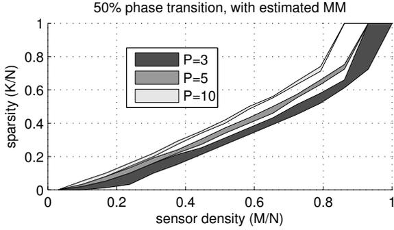
**Fig. 2.** Experimental performance of MMV with estimated MM. Each shaded area comprises all the 50% phase transitions for noise levels ranging from 0% to 10%. MMV is seen to be much robust to the presence of noise.
