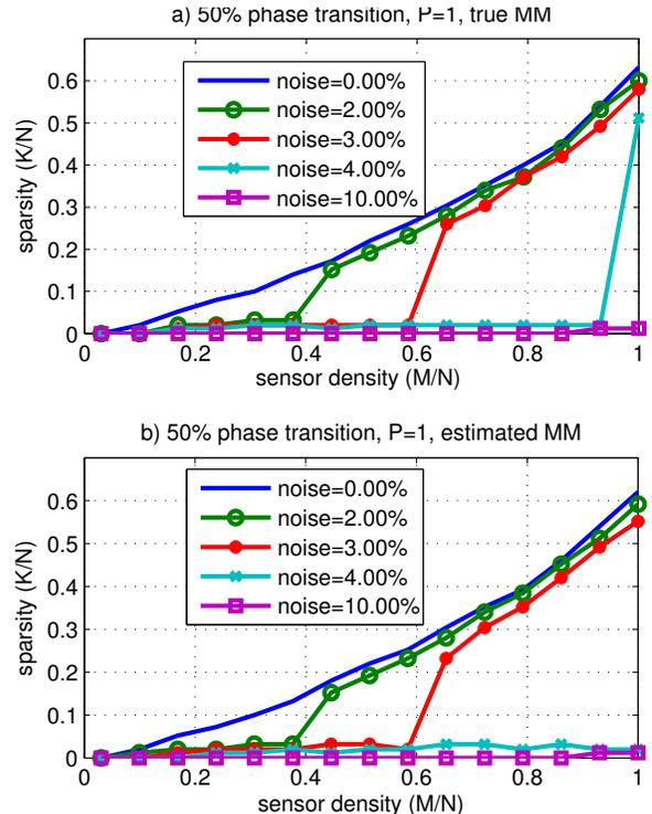
**Fig. 1.** Experimental 50% phase transitions of OMP-SMV with a) True MM and b) Estimated MM, at different levels of noise. Performance drop at 3% of noise. The  $(M, N)$  configurations below (above) each curve correspond to success (failure), respectively.
