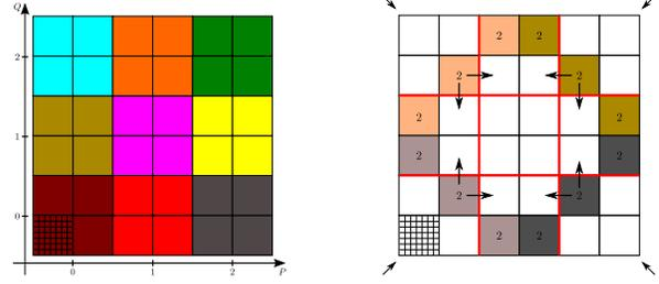
(a) Illustration of the blocked data distribution. MacroCells of similar colors belong to the same process. (b) Simultaneous sweep of all quadrants. This shows that in this example  $M_2$  is equal to 2.
