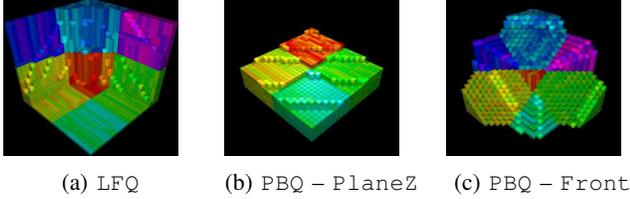
Figure 6: Snapshots showing the behaviour of various scheduling strategies on the sweep progress throughout the spatial domain. Data is distributed over a  $2 \times 2 \times 2$  process grid, and threads belonging to the same node have similar colors.
