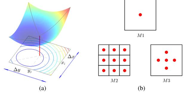
Figure 3. (a) Illustration of the value of  $V_{nm}$  over the mapped region of size  $\Delta x \times \Delta y$ . (b) Some approximation schemes for numerical integration of 2D functions over a square region. The red dots represent the sampling locations.
