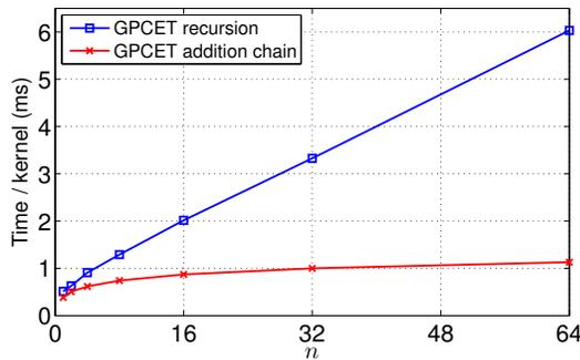
Figure 12. GPCET kernel computation times at different values of  $n$  by using recursive and addition chain-based computation.
