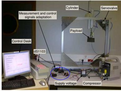
Fig. 3. Experimental setup
