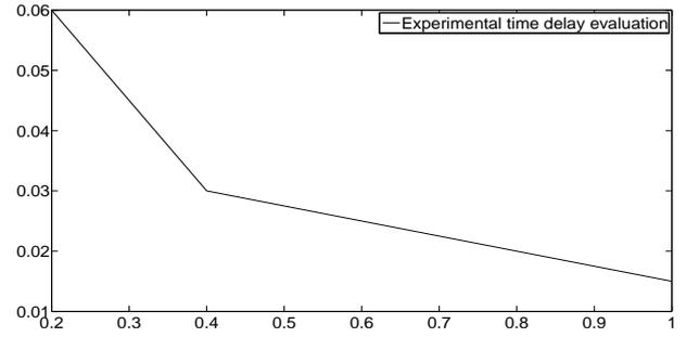
Fig. 1. Time delay (second) versus percentage of servovalve opening
