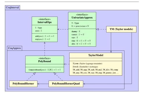
**Fig. 3** Diagram (UML) that summarizes the architecture of the CoqApprox package w.r.t. CoqInterval. The three kinds of arrows involved in the figure are:
