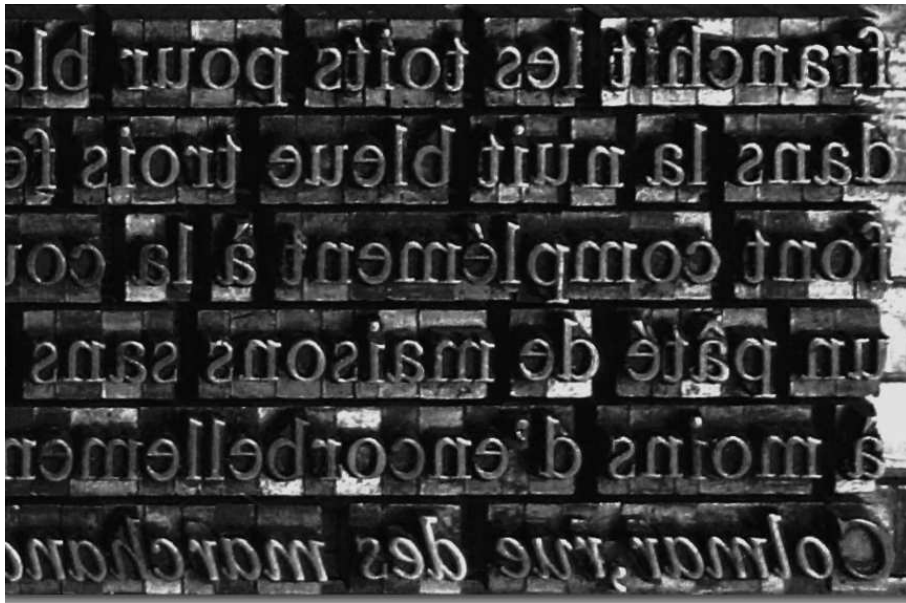
Figure 2. A picture of a movable type, set in a printing matrix and showing the alignment of the Case Height . Here, a lead Times New Roman originally created by Stanley Morison in 1932 for Monotype.
