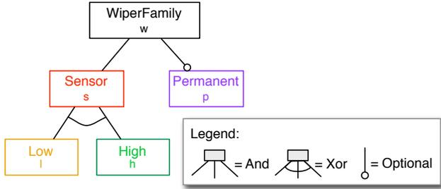
Figure 1: FD of a windscreen wiper controller SPL.
