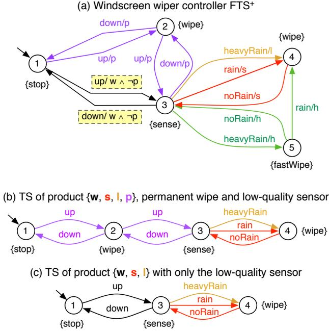
Figure 2: FTS<sup>+</sup> of the wiper controller SPL.
