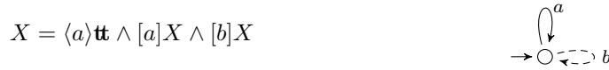
Figure 3: \nu -calculus formula and DMTS for the invariance property “there is always an ‘a’ transition available”, over the alphabet \Sigma = \{a, b\}
