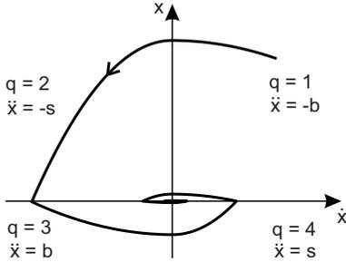
Fig. 2. Phase portrait of the twisting hybrid automaton
