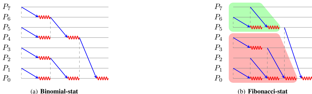
Figure 2. Schedules for Binomial-stat of order 3 and Fibonacci-stat of order 4, both using 8 processors. For Fibonacci-stat , the two schedules of order 2 and 3 used in the recursive construction are highlighted in green and red.
