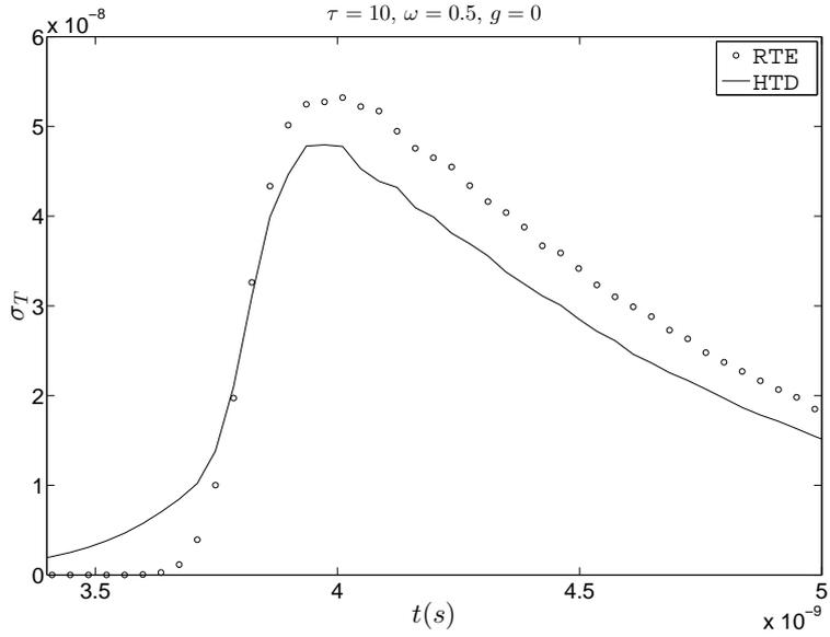
Figure 7: MCM solutions of the RTE and the HTD models. Time history of the dimensionless transmittance (a), and of the statistical uncertainties (b) for an optical thickness  $\tau = k_a + k_s = 10$ , an albedo  $\omega = 0.5$ , and an isotropic phase function.
