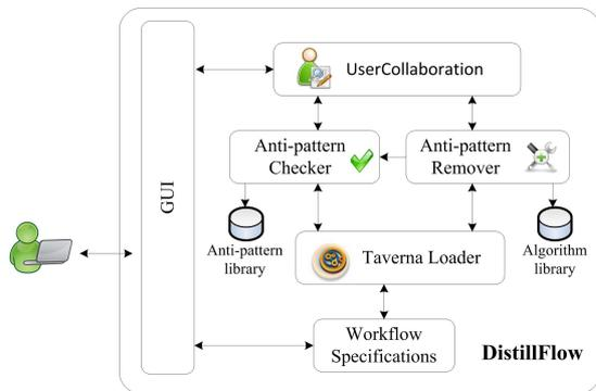
Figure 3: Architecture of DistillFlow
