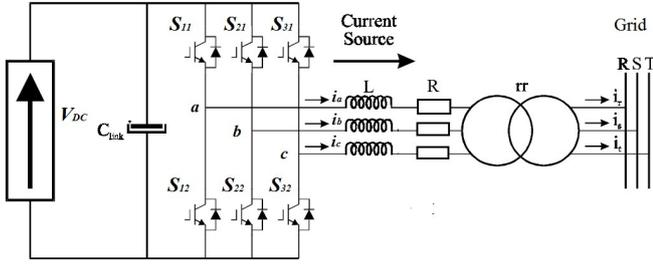
Fig. 5. Two-level voltage source inverter circuit topology.
