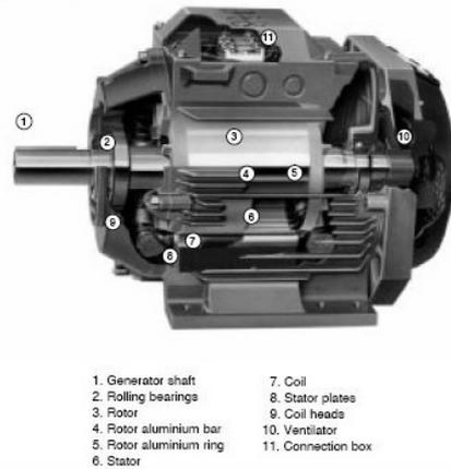
Fig. 4. Cutaway of a squirrel-cage induction generator.
