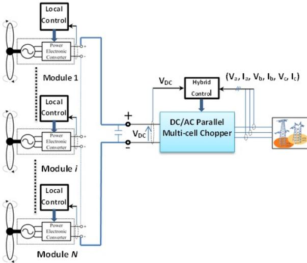
Fig. 2. Chain of production of wind energy.
