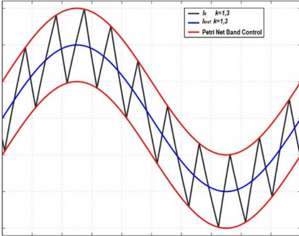
Fig. 7. Strategy of control using a hysteresis-type controller.
