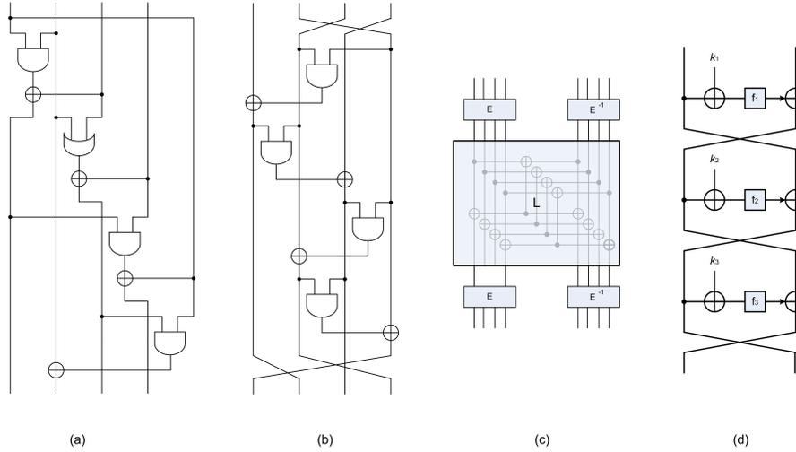
**Fig. 1.** (a) Non involutive 4-bit S-box with optimal bitslice representation. (b) Involutive 4-bit S-box with optimal bitslice representation. (c) Construction of 8-bit S-boxes from 4-bit ones as in the Whirlpool hash function [44]. (d) Construction of  $2s$ -bit S-boxes from  $s$ -bit ones as in the MISTY block cipher [36].
