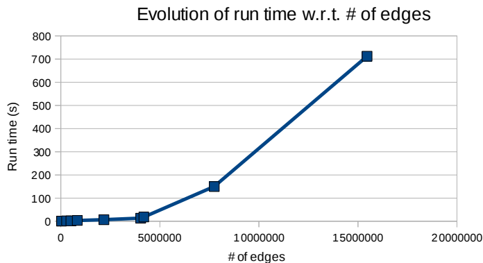
Figure 8: Evolution of run times with respect to # of edges in an alignment graph of 21904 vertices.
