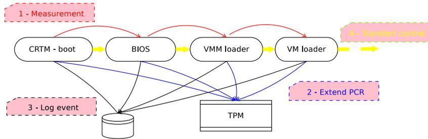
**Fig. 3.** State-of-Art of a complete secure boot chain.
