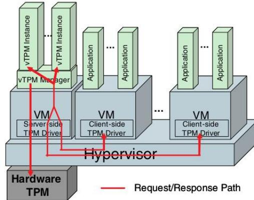
Fig. 5. The mostly implemented solution in para-virtualized hypervisors [22].
