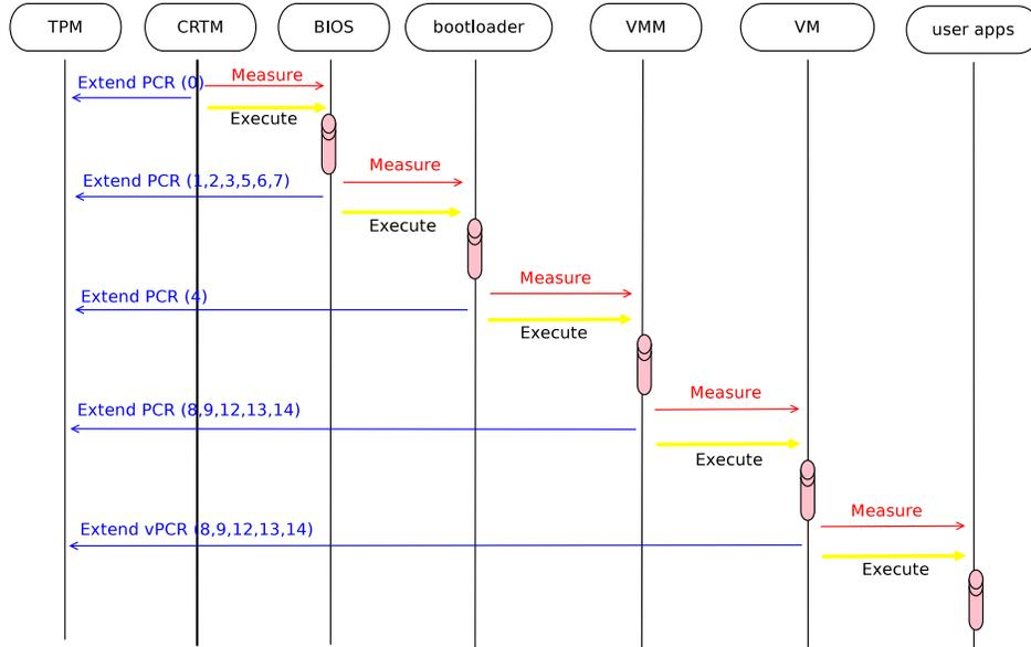
**Fig. 7.** measured boot: measuring, launching, reporting
