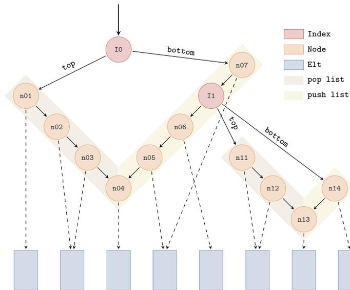
Figure 6: Example of a possible queue internal structure. Here, the main queue is accessible through the index  $I_0$ . The index  $I_1$  is pointing to a queue concatenated during a previous merge operation. This queue will be unfolded during the next normalization. Because of the Irmin store behavior, two nodes containing the same element share its physical representation.
