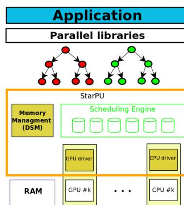
**Fig. 1** The architecture of the StarPU runtime system.
