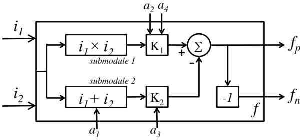
Fig. 1. Block diagram of configurable logic unit.
